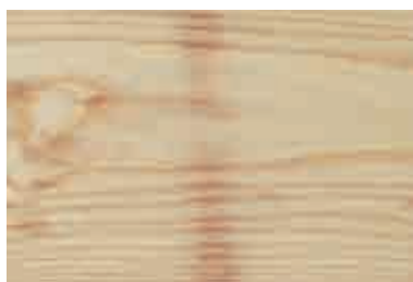
STICKER STAIN: Stain that is typically grey in colour occurring from stickers used to season lumber.
