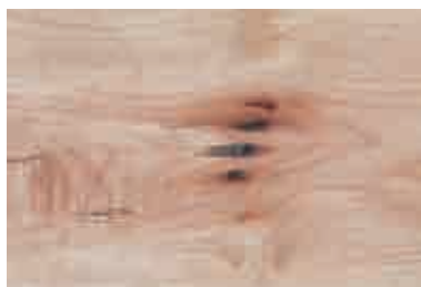
BIRD PECKS: Small blemishes in the grain pattern resulting from birds pecking that sometimes contain ingrown bark. An exception to the rule is hickory and elm.
