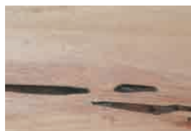
GRUB HOLES: Holes larger than \frac{1}{4} "
